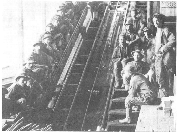
These cramped cable car skips were how the miners were taken into the mines and brought back to the surface. The collar of the mine is the surface entrance to the mine shaft. Each miner was paid, "collar to collar," four to five dollars per 8-hour day. Photo courtesy Empire Mine State Historic Park.
