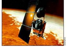
The units mismatch prevented navigation information from transferring between the Mars Climate Orbiter spacecraft team in at Lockheed Martin in Denver and the flight team at NASA's Jet Propulsion Laboratory in Pasadena, California.
