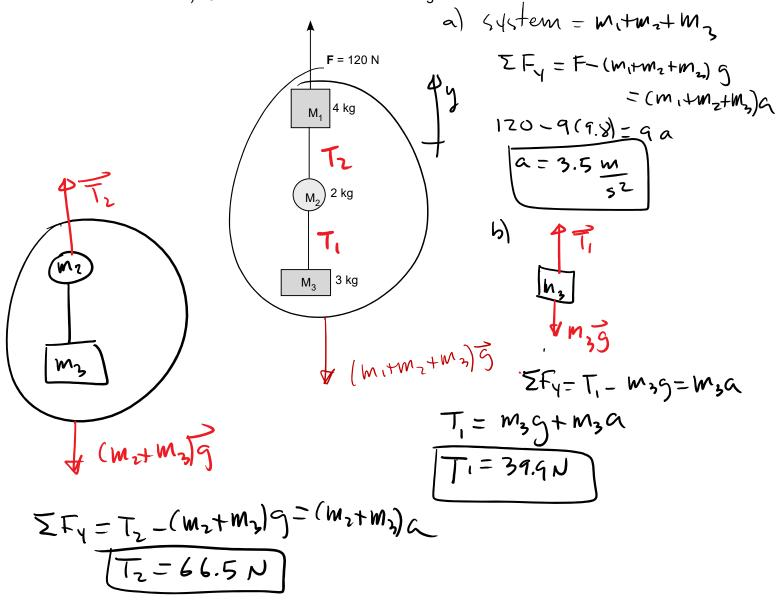
2. For the system shown below, calculate the force the 3-kg block exerts on the 2kg block. Assume masses move on a frictionless surface. (10 pts)
