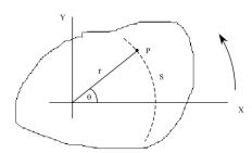
As the body rotates the particle moves in a circular path of radius 'r'. The distance the particle moves along this path is related to its angular position ' $\theta$ ' by the equation:
